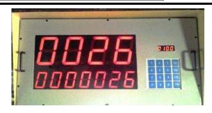
The instrument is single Microcontroller based, SWITCH MODE POWER SUPPLY UNIT (SMPS), KEYPAD for programming & counter setting & resetting, seven segment display unit for displaying running COUNT, TOTALIZER, SET/PRESET COUNT. Use of HIGHLY DURABLE SENSING HEAD instead of conventional optical sensors & proximity switches gives better results, longer life in dusty (CEMENT INDUSTRY) and rough industrial atmosphere. The unit comes with 3 display:-
